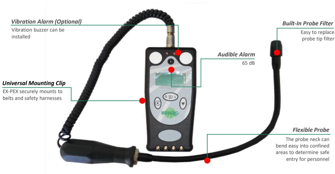
EX-PEX with Flexible Detection Probe
